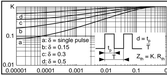
Fig.2 Typical transient thermal impedance
