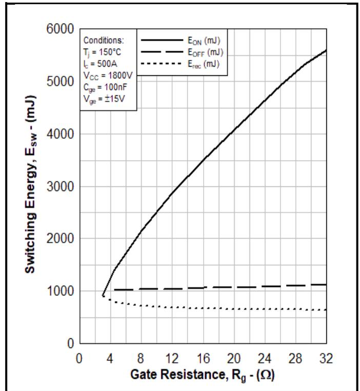
Fig. 6 Typical switching energy vs gate resistance
