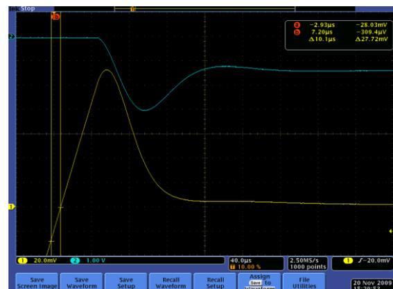
Fig.5 Reverse recovery waveforms
