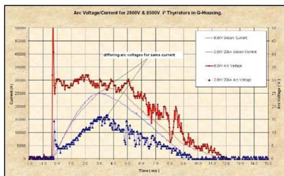
**Fig. 3 Reverse fault current and arc voltage.**
