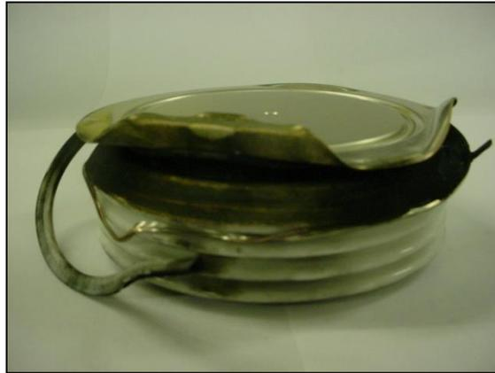
**Fig. 9 Thyristor with arc shield finally failing at the cold-weld due to internal pressure.**
