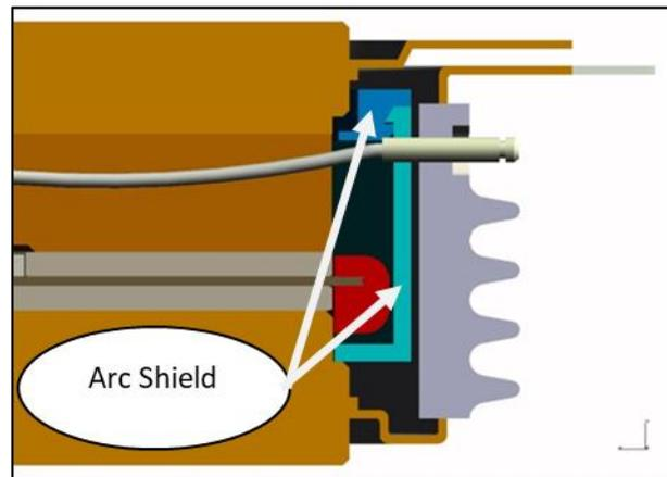
**Fig. 6 Schematic diagram of arc shield design.**
