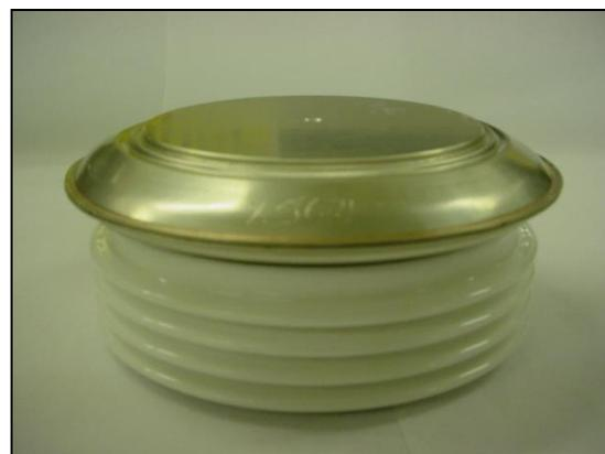
**Fig. 8 Device with arc shield after test at higher current than in fig. 7 with increased swelling due to internal pressure.**
