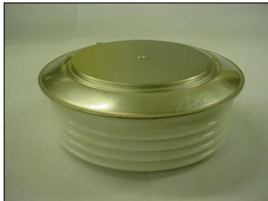
**Fig. 7 Device with arc shield after test starting to swell due to internal pressure.**
