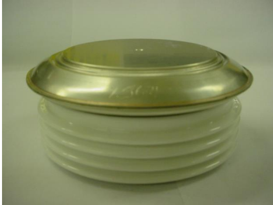
Figure 8. Device with arc shield after test at higher current than in Fig 7 with increased swelling due to internal pressure.
