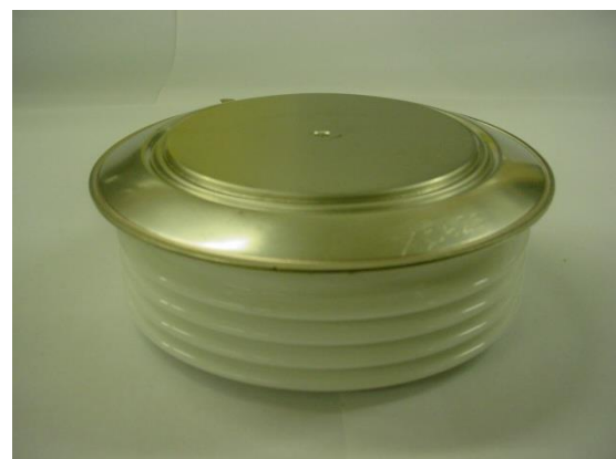
Figure 7. Device with arc shield after test starting to swell due to internal pressure.
