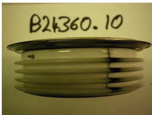
Fig 5. Thyristor after test showing cracked ceramic due to thermal shock
