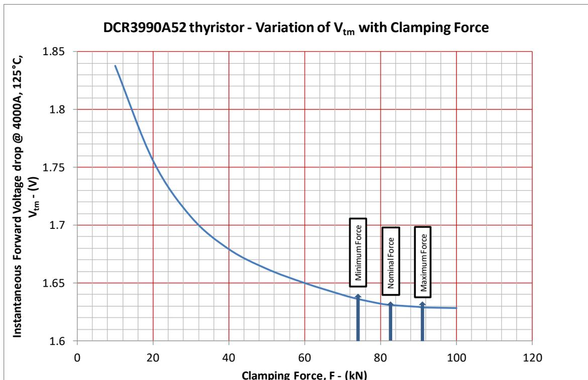
Figure 3: DCR3990A52 thyristor – variation of Forward Voltage Drop with clamping.
