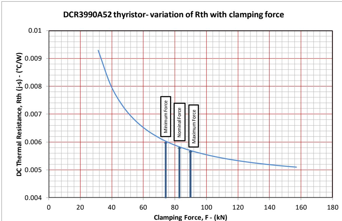
Figure 2: DCR3990A52 thyristor – variation of thermal resistance with clamping force.
