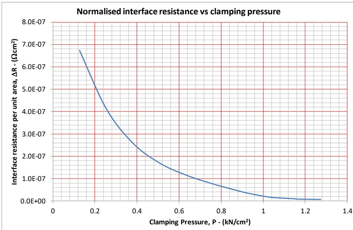
**Figure 4: Normalised interface resistance variation with clamping pressure.**
