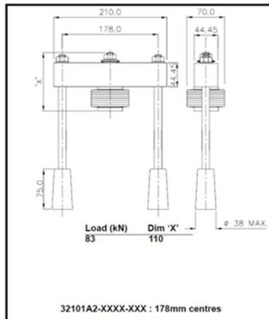
Figure 5: Typical Clamp for Double Side Cooling.
