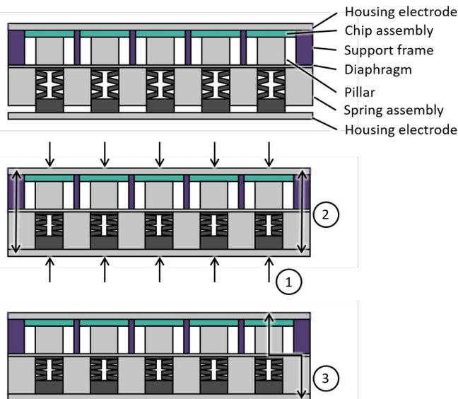
Figure 3: Illustration of the DLB (a) unclamped state, (b) clamped state, (c) current path.
