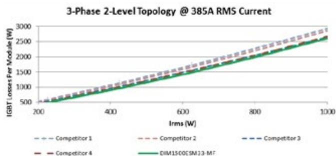
Figure 1: 3-Phase 2-Level Topology @ 385A RMS Current
