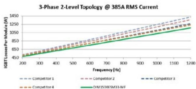
Figure 2: 3-Phase 2-Level Topology @ 385A RMS Current
