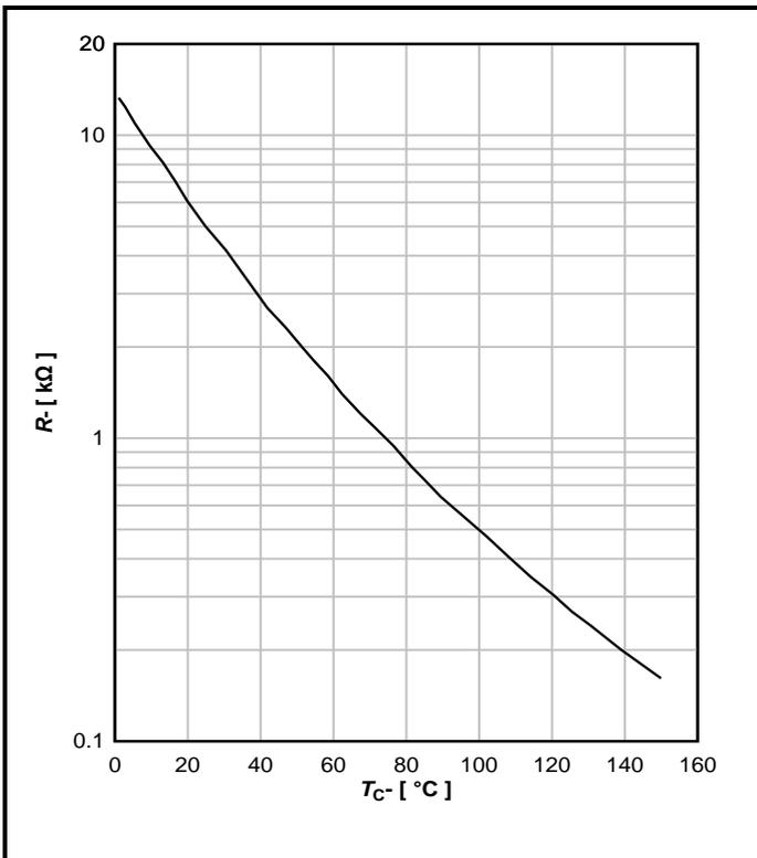
Fig. 17 Typical NTC thermistor characteristics
