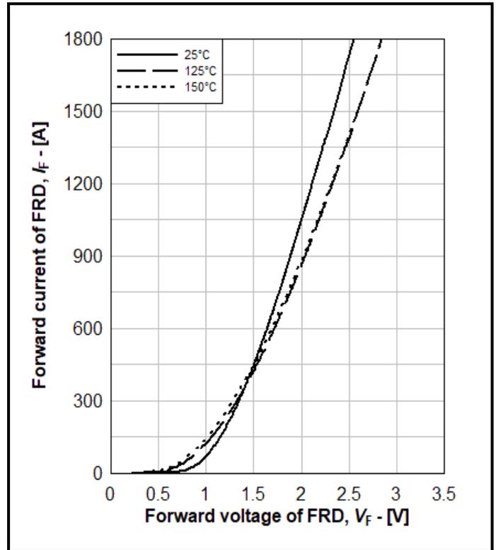
Fig. 12 Typical FRD output characteristics
