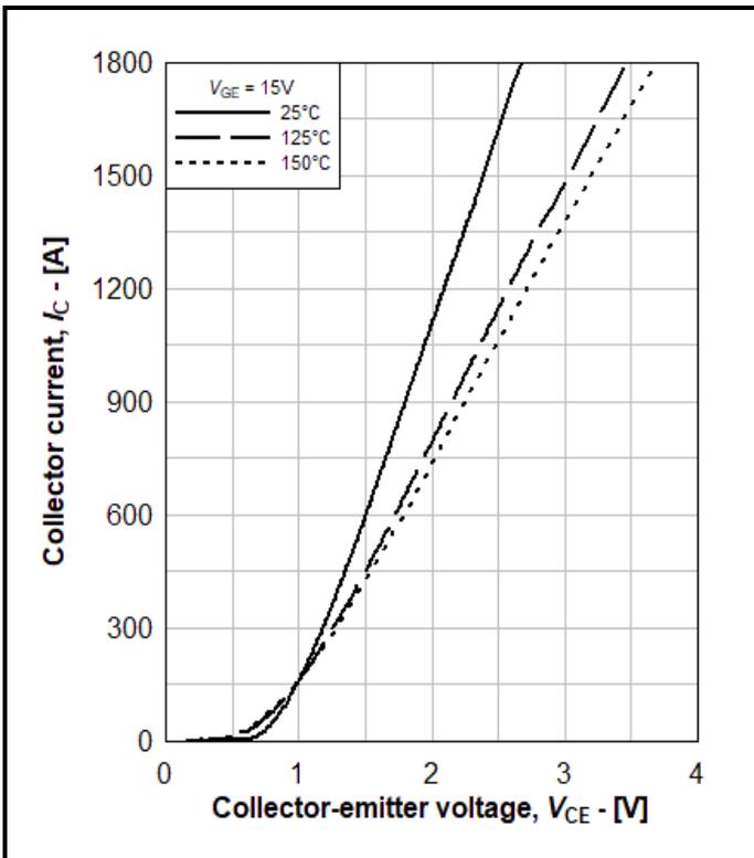
Fig. 5 Typical IGBT output characteristic
