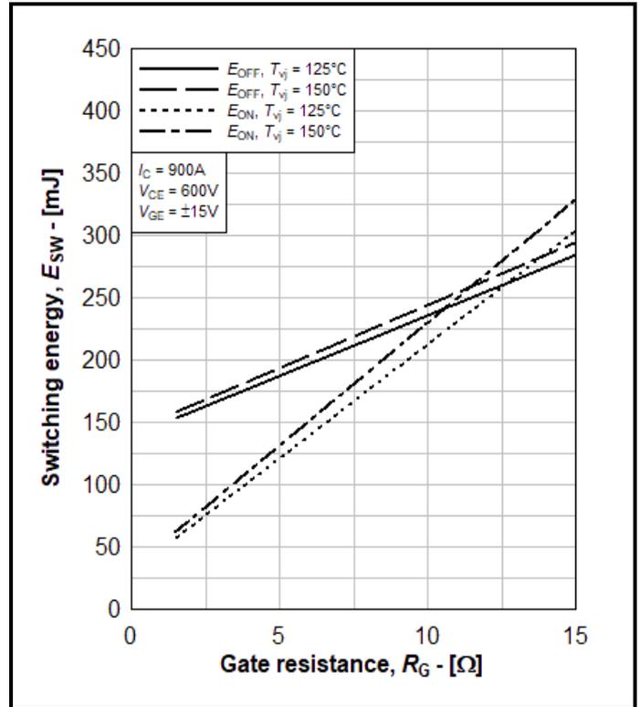
Fig. 8 Typical IGBT switching energy
