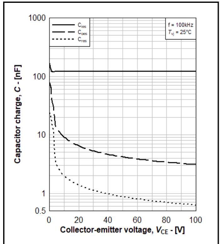
Fig. 10 Typical capacity characteristic
