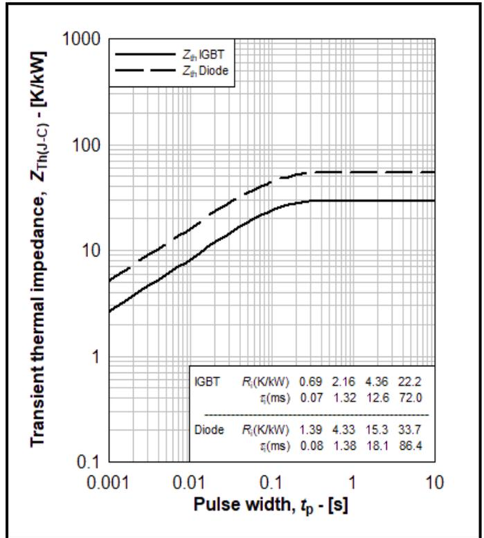
Fig. 16 Transient thermal impedance
