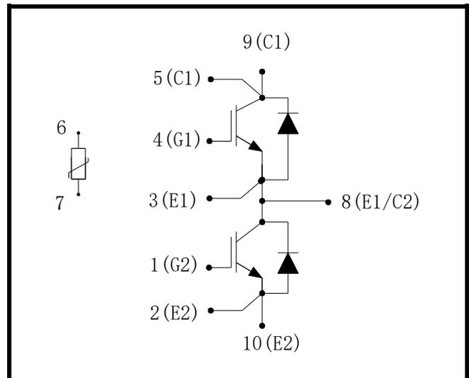
**Fig. 1 Circuit configuration**
