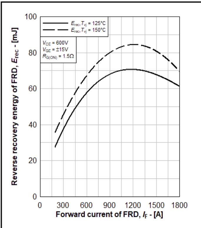
Fig. 13 Typical FRD switching loss
