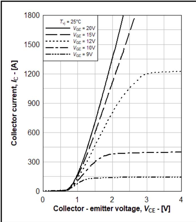
Fig. 3 Typical IGBT output characteristic
