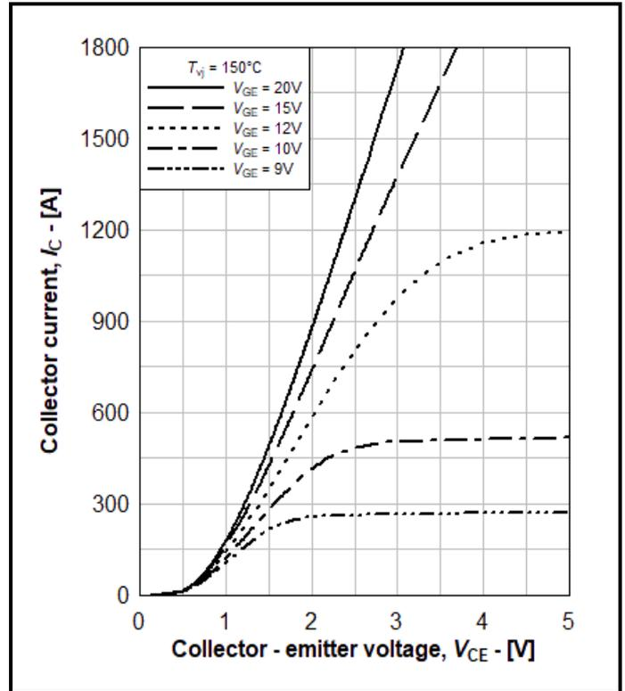
Fig. 4 Typical IGBT output characteristic
