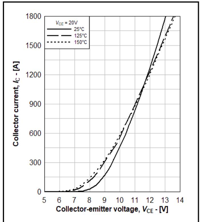
Fig. 6 Typical IGBT transfer characteristic
