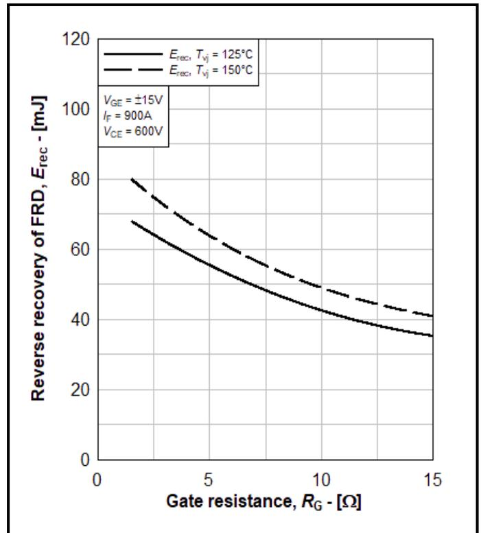
Fig. 14 Typical FRD switching loss
