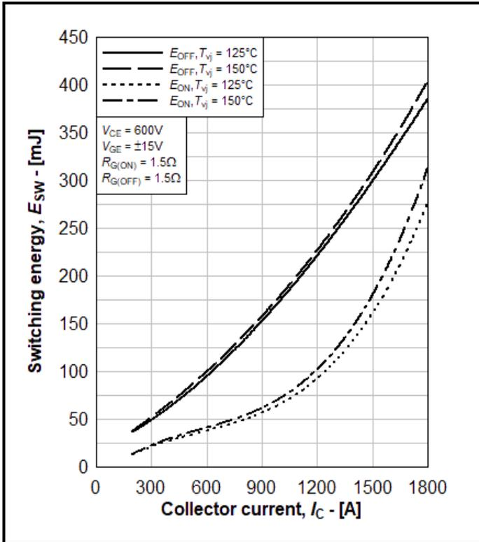
Fig. 7 Typical IGBT switching energy
