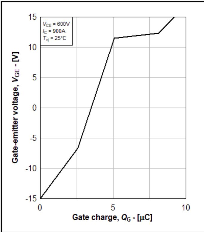
Fig. 11 Typical gate charge characteristic
