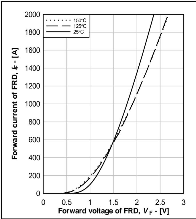
Fig. 7 Diode typical forward characteristics,  $I_F = f(V_F)$
