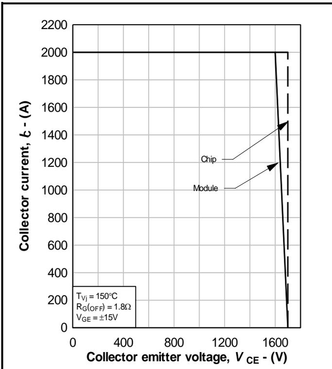
Fig. 13 Reverse bias safe operating area of IGBT,
