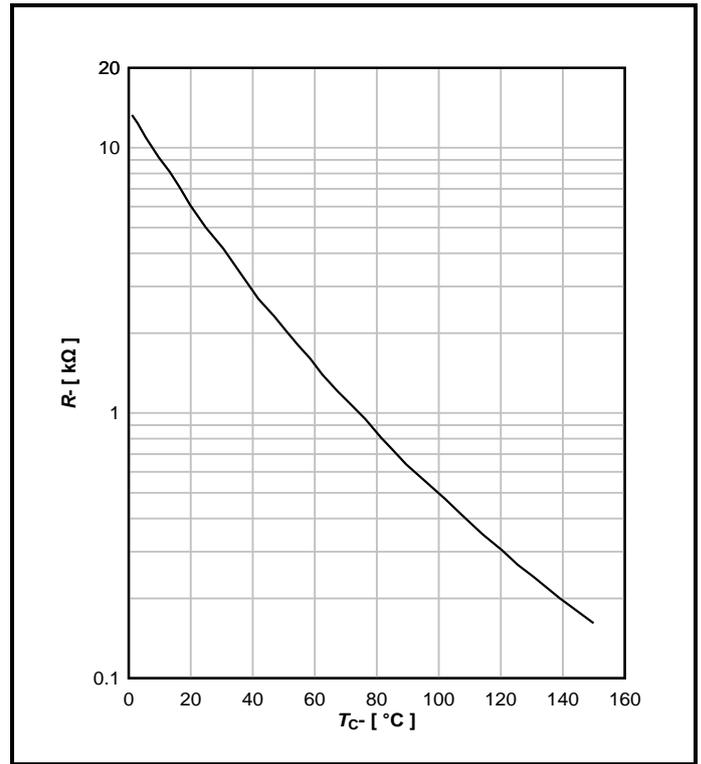
Fig. 12 Typical NTC thermistor characteristic,  $R = f(T_C)$
