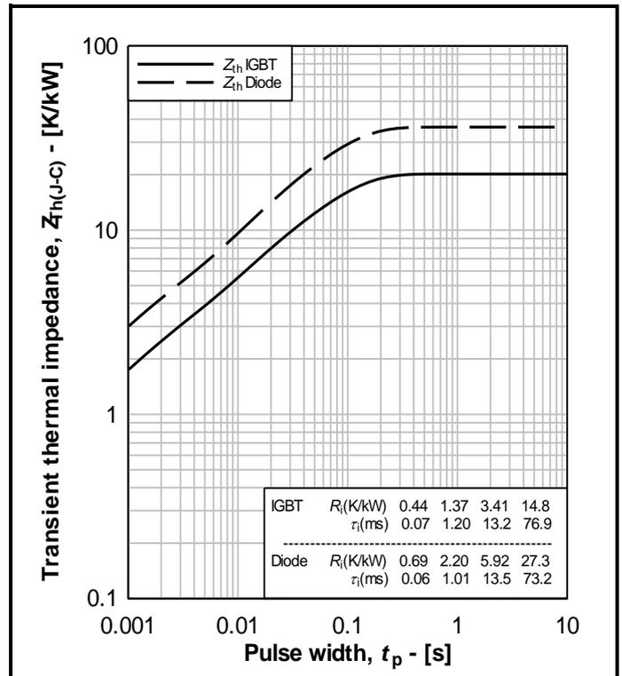
Fig. 14 Transient thermal impedance,  $Z_{th(J-C)} = f(t)$
