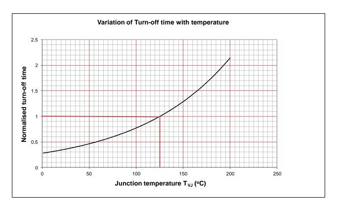
The graphs for the variation in turn-off time with temperature, re-applied voltage and di/dt can be combined into an EXCEL spreadsheet to estimate the turn-off time under conditions different to the datasheet conditions
