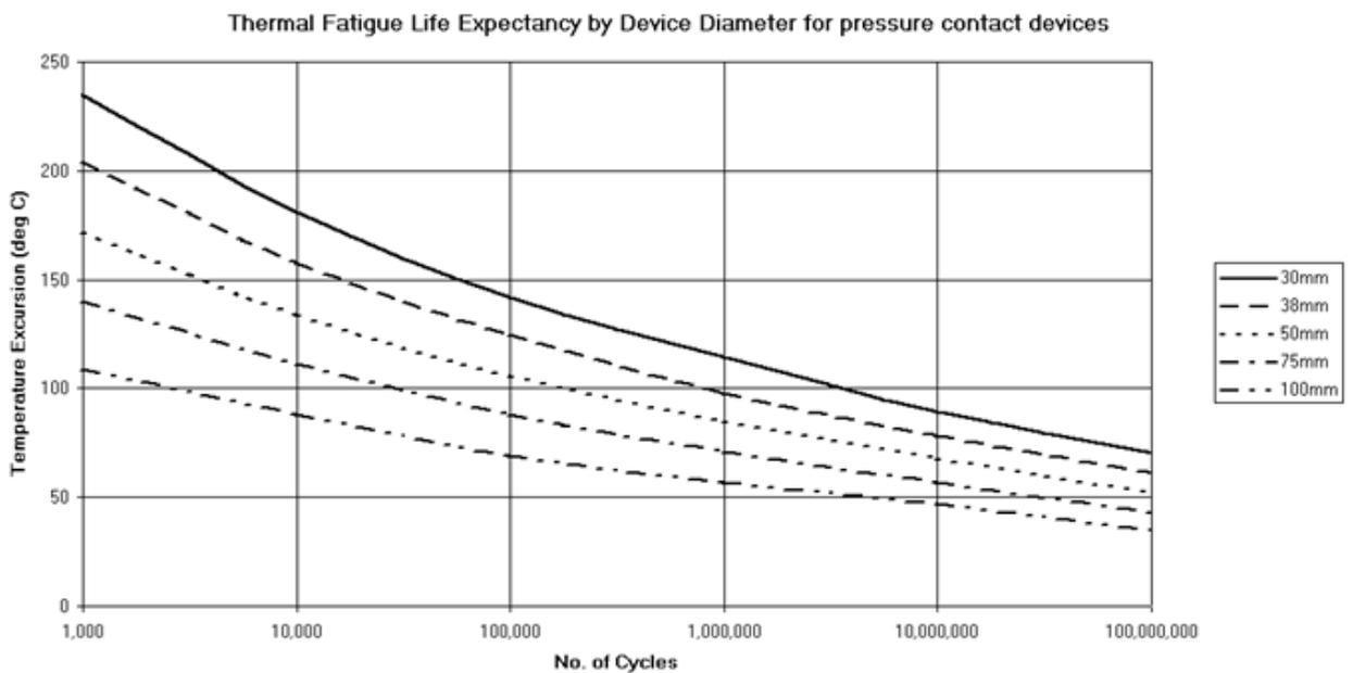
**Fig. 5 Thermal fatigue life failure**
