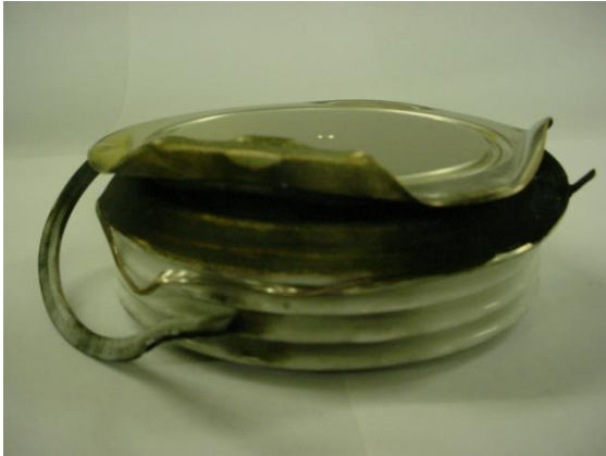
Fig. 8. Thyristor with arc shield finally failing at the cold weld due to internal pressure.
