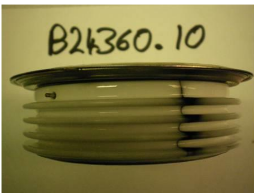
Fig 5. Thyristor after test showing cracked ceramic due to thermal shock
