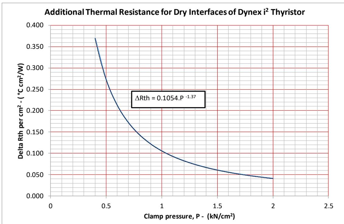
**Figure 1 Thermal resistance of dry interfaces of a fully floating thyristor.**
