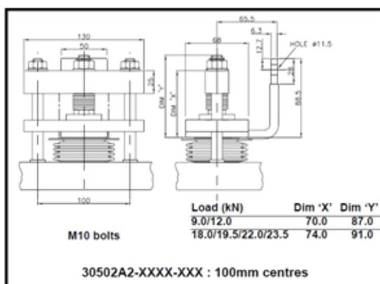
**Figure 6 Typical Clamp for Single Side Cooling**
