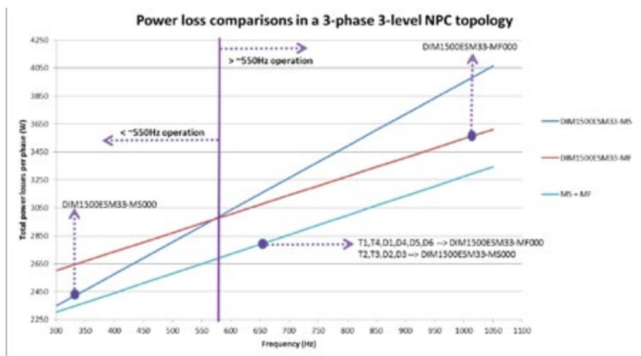
Figure 2a: Semiconductor Power losses per phase (W) Vs. Frequency (Hz) MS vs MF and optimised use of MF + MS
