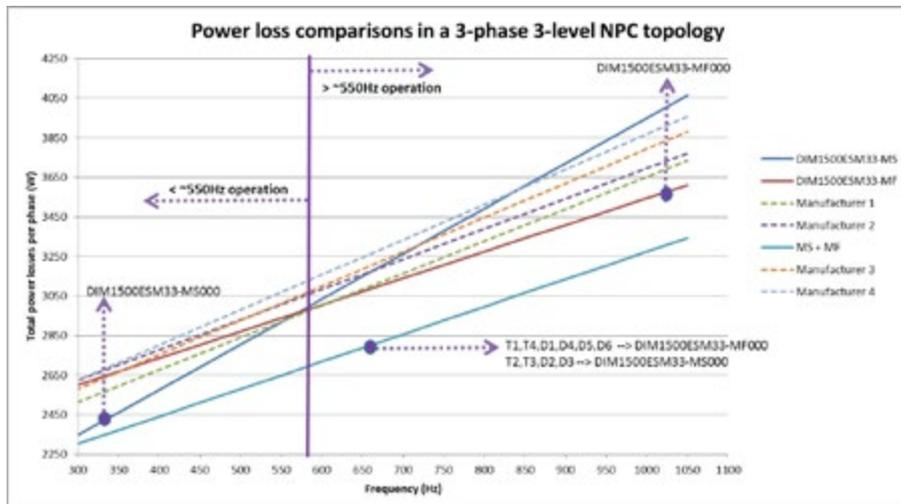
Figure 2b: Comparison of Power Losses using Dynex MS and MF variant modules vs modules from four competitors.
