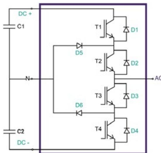
Figure 1: Content of a 3L NPC Phase Leg
