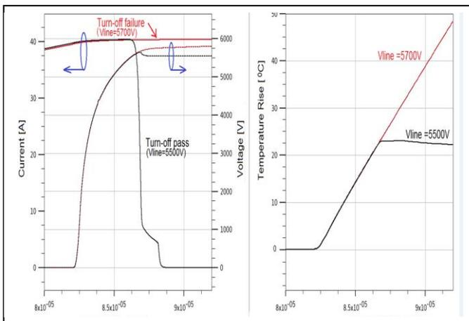
**Fig.5:** Electro-thermal simulation with baseplate temp=125°C showing successful turn-off at  $V_{line}=5500V$  and failure at 5700V. Whilst the device temperatures start reducing after successful turn-off, it keeps increasing with failure.
