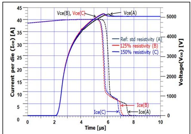
**Fig7:** Simulated turn-off  $I_{ce}$  and  $V_{ce}$  waveforms for different n-base resistivity
