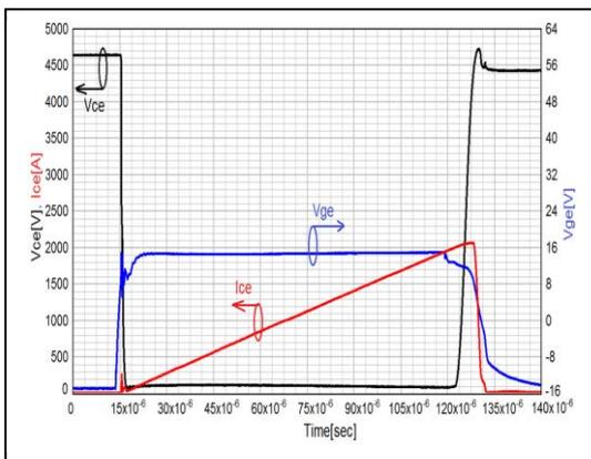
**Fig.3:** Measured succesful  $I_{ce}=2000A$  turn-off at  $V_{line}=4600V$ ,  $T=150^{\circ}C$ ,  $V_{ge}=\pm 15V$ ,  $C_{ge}=330nF$ ,  $R_{goff}=15\Omega$ ,  $L_s=200nH$
