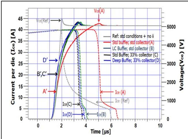
**Fig.6:** Simulated turn-off  $I_{ce}$  and  $V_{ce}$  waveforms for different buffer and collector designs (A-D) compared with ideal case of standard structure where impact ionization is turned off. Arrows A-D indicates the onset of dynamic avalanche, when  $V_{ce}$  slope becomes less than that of  $V_{ce}(ref)$ .  $V_{line}=5kV$ ,  $I_{ce}=42A$ ,  $R_{goff}=8\Omega$ ,  $T=25^{\circ}C$
