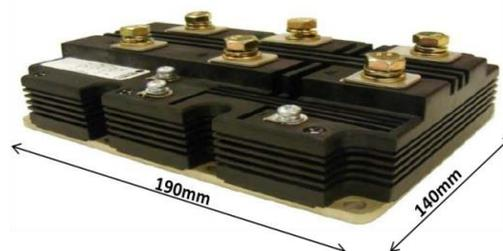
**Fig.1:** Device under test: The 6.5kV/1000A Trench gate IGBT module in the 190mm x 140mm footprint.
