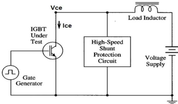
**Fig.2:** Test circuit for analysis of IGBT Turn-off. The DUT(Device Under Test) is unclamped.
