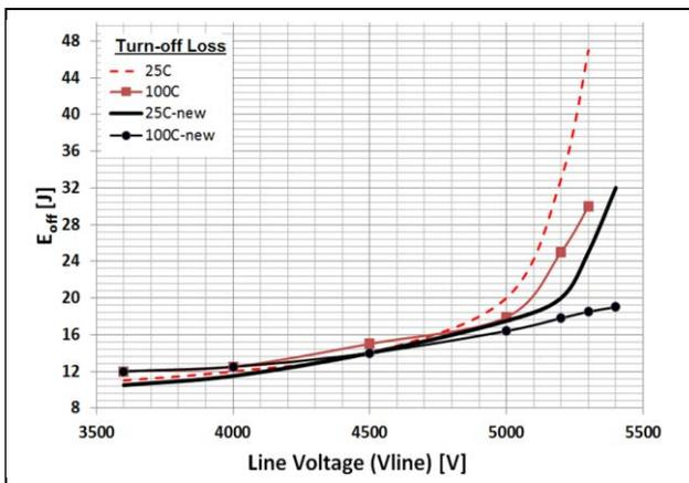
**Fig.9:** Comparison of measured  $E_{off}$ - $V_{line}$  curves for old and new optimized modules.  $I_{OFF}=1000A$ .
