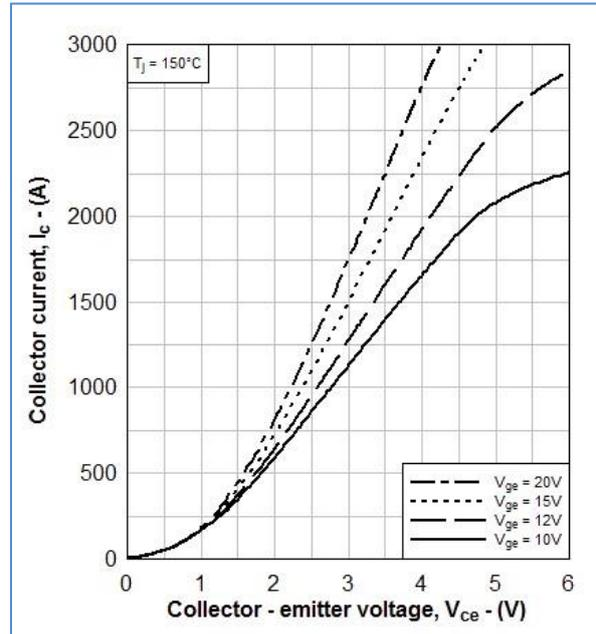
Figure 4: Typical output characteristics Tj @ 150°C
