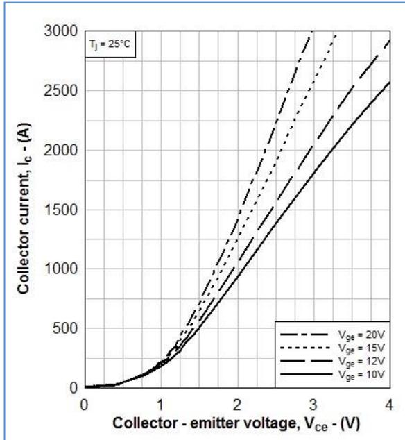
Figure 3: Typical output characteristics Tj @ 25°C
