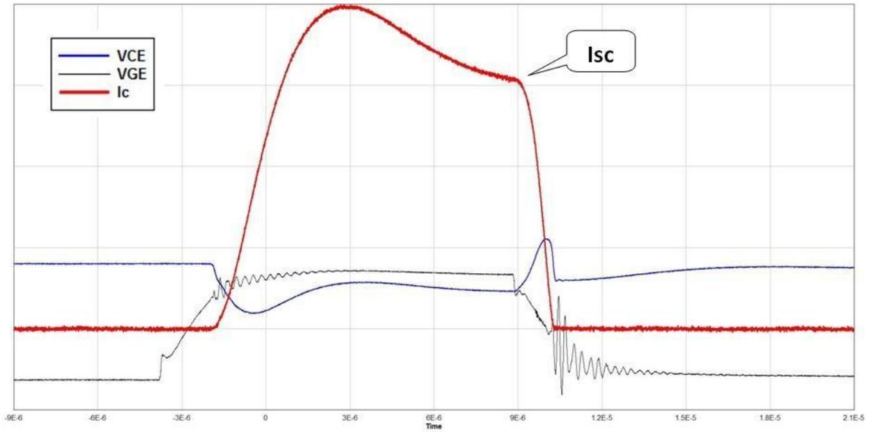
Figure IV: Short Circuit Current ISC
