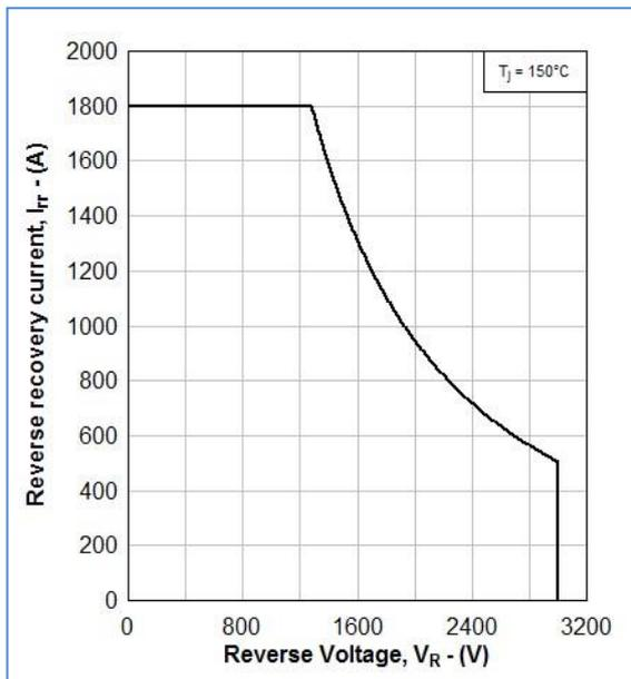
Figure 9: Diode reverse bias safe operating area
