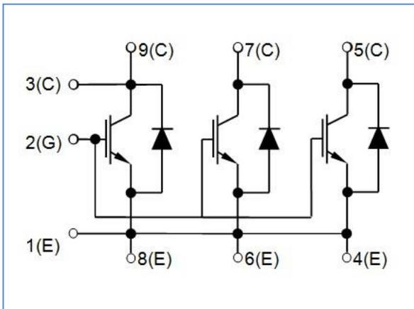
**Figure 1: Circuit configuration**
