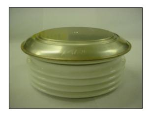
Fig. 8 Device with arc shield after test at higher current than in fig. 7 with increased swelling due to internal pressure.
