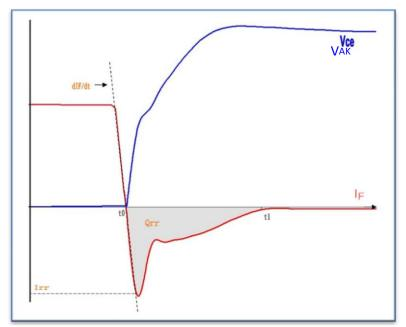
Figure II: Diode timing diagram
