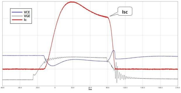
Figure IV: Short Circuit Current ISC
