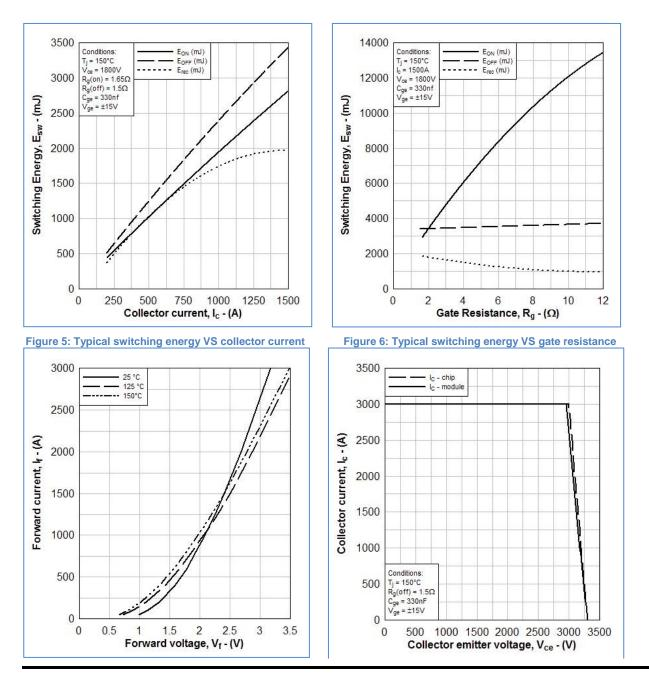
Figure 7: Diode typical forward characteristics
