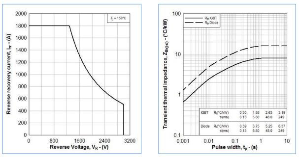
Figure 9: Diode reverse bias safe operating area
