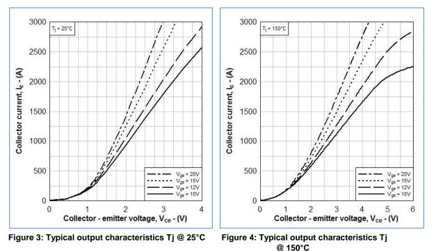
This is one of the key parameters of the IGBT and it is used to calculate on-state power loss in the IGBT. The average conduction power loss  $P_{avg(cond)}$  in the IGBT is given by:
