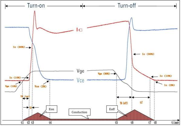
Figure I: Timing diagram and energy losses
