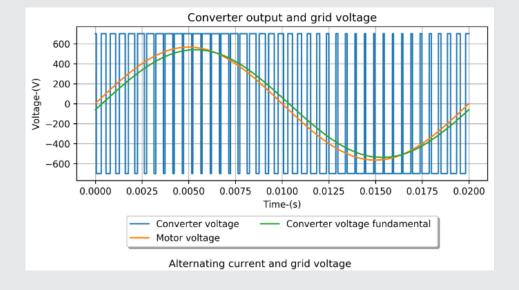
The values for alternating current, grid voltage and current in phase 1 are displayed graphically.
