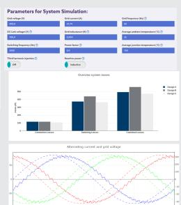
The instantaneous and average power losses in each semiconductor component of the circuit are displayed for each topology, selected alongside other outputs shown below.
