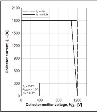
Fig. 9 Reverse bias safe operating area of IGBT
