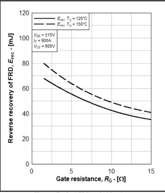
Fig. 14 Typical FRD switching loss
