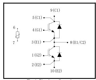
Fig. 1 Circuit configuration
