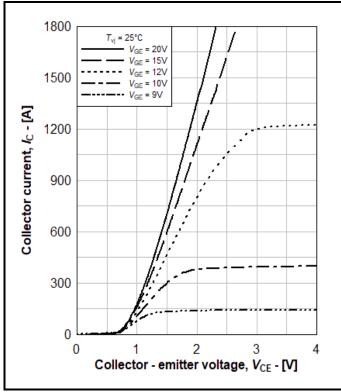
Fig. 3 Typical IGBT output characteristic
