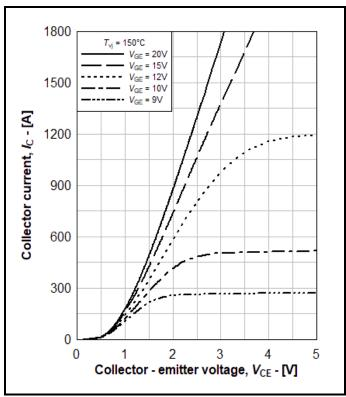
Fig. 4 Typical IGBT output characteristic
