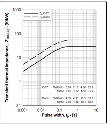
Fig. 16 Transient thermal impedance
