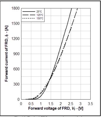
Fig. 12 Typical FRD output characteristics
