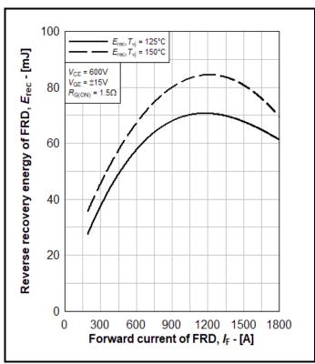
Fig. 13 Typical FRD switching loss
