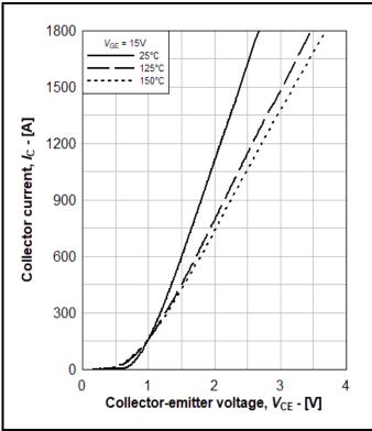
Fig. 5 Typical IGBT output characteristic
