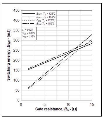
Fig. 8 Typical IGBT switching energy
