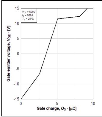
Fig. 11 Typical gate charge characteristic
