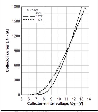
Fig. 6 Typical IGBT transfer characteristic
