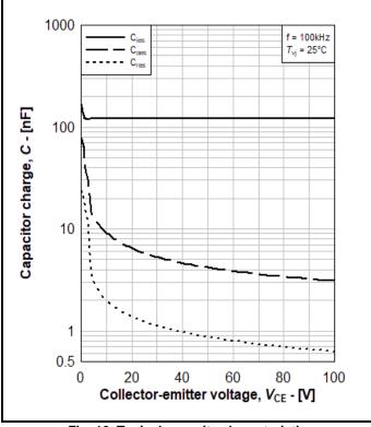
Fig. 10 Typical capacity characteristic
