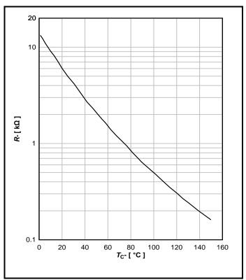
Fig. 17 Typical NTC thermistor characteristics
