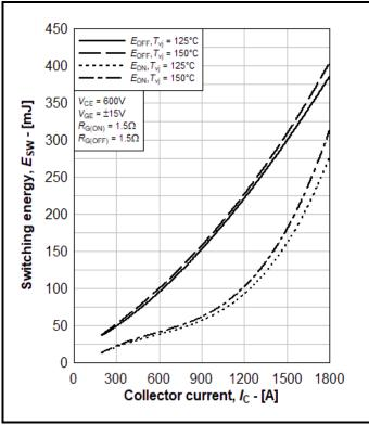
Fig. 7 Typical IGBT switching energy
