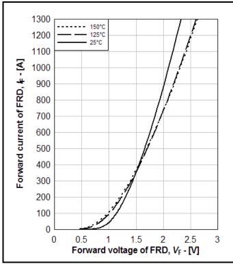
Fig. 7 Diode typical forward characteristics
