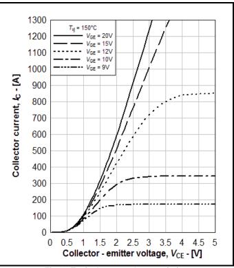
Fig. 4 Typical output characteristics
