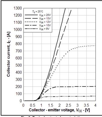
Fig. 3 Typical output characteristics
