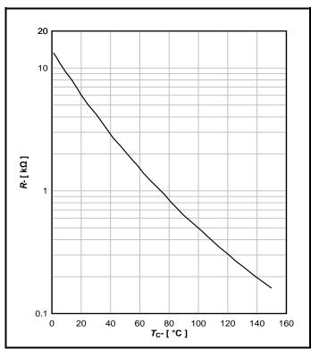
Fig. 9 Typical NTC thermistor characteristics
