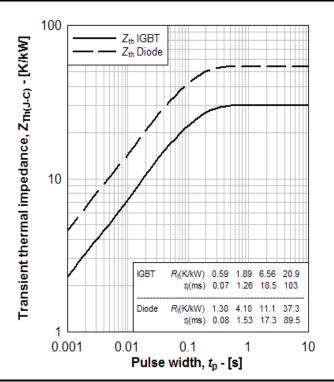
Fig. 10 Transient thermal impedance
