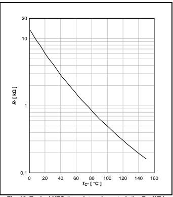
Fig. 12 Typical NTC thermistor characteristic,  $R = f(T_C)$
