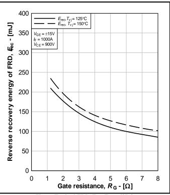
Fig. 8 Typical FRD  $E_{rec}$ ,  $E_{rec} = f(R_G)$
