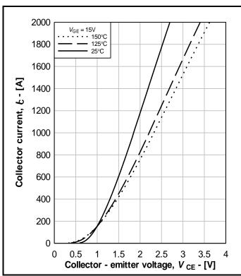
Fig. 5 Typical IGBT output characteristics,  $I_C = f(V_{CE})$
