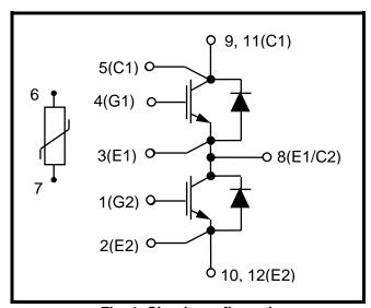
Fig. 1 Circuit configuration
