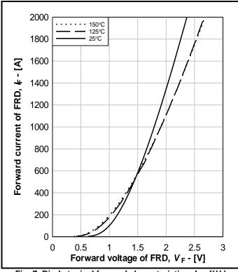
Fig. 7 Diode typical forward characteristics,  $I_F = f(V_F)$
