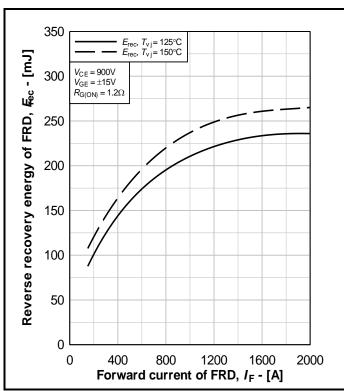
Fig. 9 Typical FRD  $E_{rec}$ ,  $E_{rec} = f(I_F)$
