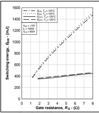
Fig. 11 Typical IGBT switching energy  $E_{ON} = f(R_G)$ ,  $E_{OFF} = fR_G$ )
