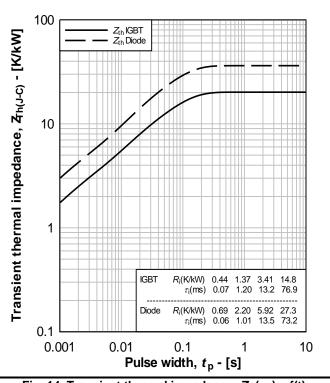
Fig. 14 Transient thermal impedance,  $Z_{th}(J-C) = f(t)$
