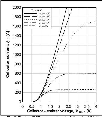
Fig. 3 Typical IGBT output characteristics,  $I_C = f(V_{CE})$
