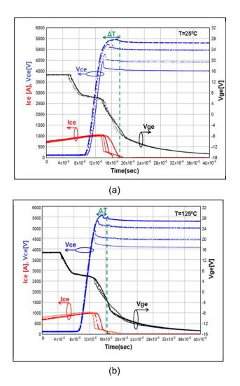
**Fig.8a-b**: Measured waveforms of optimised module for increasing Vline turn-off at **a**)  $25^{0}$ C and **b**)  $100^{0}$ C.  $\Delta$ T is the increase in turn-off delay time due to avalanche SSCM period at 5.3kV. Vline=3.6-5.3kV, Vg=±15V, I<sub>OFF</sub>=1000A, Ls=200nH, Cge=330nF, R<sub>goff</sub> =15 $\Omega$
