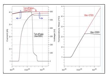
**Fig.5:** Electro-thermal simulation with baseplate temp=125<sup>o</sup>C showing successful turn-off at Vline=5500V and failure at 5700V. Whilst the device temperatures start reducing after successful turn-off, it keeps increasing with failure.
