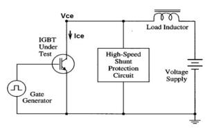
**Fig.2:** Test circuit for analysis of IGBT Turn-off. The DUT(Device Under Test) is unclamped.
