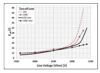
**Fig.9**: Comparison of measured  $E_{off}$ -Vline curves for old and new optimised modules.  $I_{OFF}$ =1000A.
