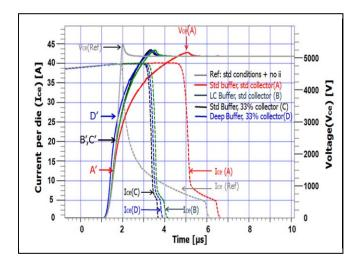
**Fig.6:** Simulated turn-off Ice and Vce waveforms for different buffer and collector designs (A-D) compared with ideal case of standard structure where impact ionization is turned off. Arrows A-D indicates the onset of dynamic avalanche, when Vce slope becomes less than that of Vce(ref). Vline=5kV, Ice=42A,  $R_{qoff}$ =8 $\Omega$ , T=25<sup>o</sup>C
