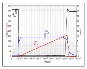
Fig.3: Measured successful Ice=2000A turn-off at Vline=4600V, T=150 $^{\circ}$ C, Vge=±15V, Cge=330nF, R<sub>aoff</sub>=15 $\Omega$ , Ls=200nH
