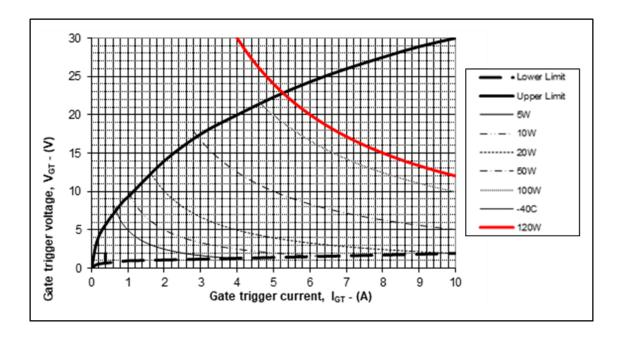
The load line of our gate drive is given by the open circuit voltage of 30V and a short circuit current of 3A. If this is plotted on the above graph it should lie to the left of the 120W peak power limit line.
