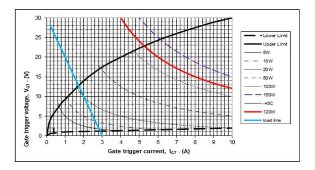
Therefore, our gate drive complies with the limit of 120W when connected to our thyristor.
