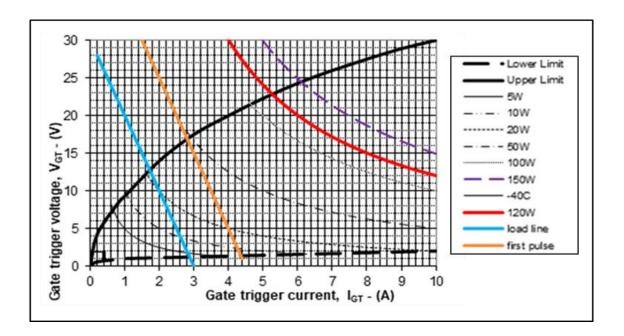
The load line is then compared to the 150W curve or the power calculated from the values of current and voltage where the load line intercepts the upper gate characteristic at 2.8A and 17V i.e. 48W. Either way, our initial gate pulse is less than 150W and our gate drive is fully acceptable from a gate power point of view.
